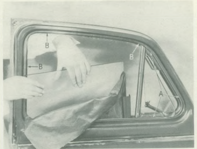
Fig. 6. Removing drop light from front door body
