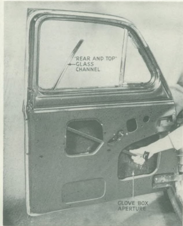
Fig. 8. Extracting "rear and top" glass channel member
