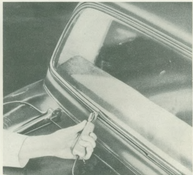
Fig. 4. Installing rubber lace with special tool
