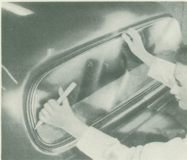
Fig. 3. Fitting glass to glazing rubber in rear light aperture
