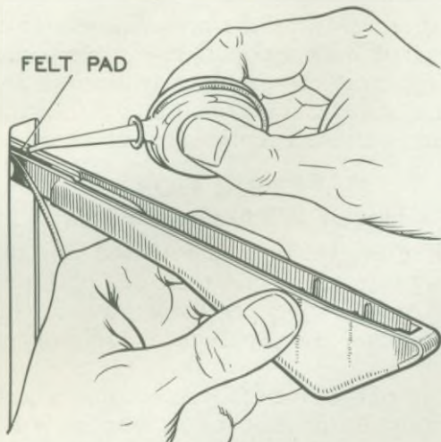
Fig. 20. Lubricating arm pivot bearing
