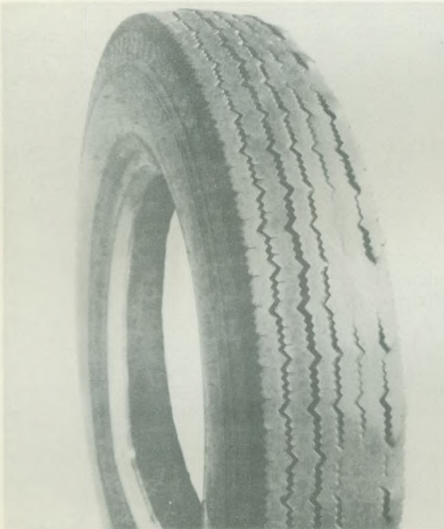
Fig. 12. Irregular spotty wear due to a variety of causes
