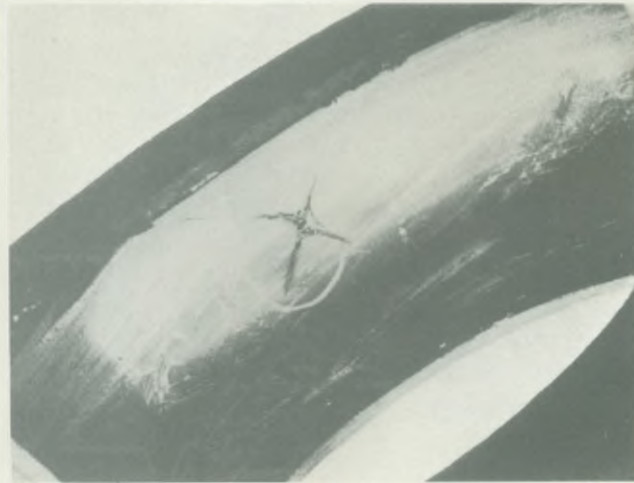
Fig. 8. Impact fracture caused by striking a sharp object such as a brick-end or pavement kerb
