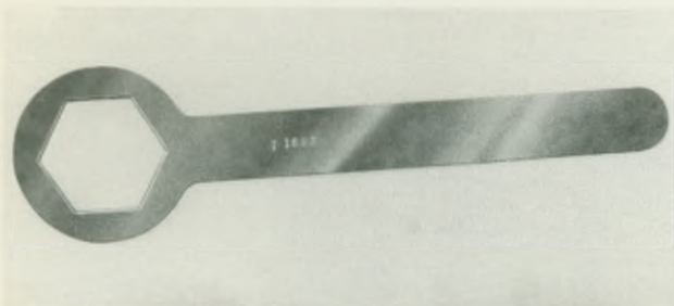
Fig. 9. Special ring spanner for removal of tapered hexagonal filler cap for Girling damper
