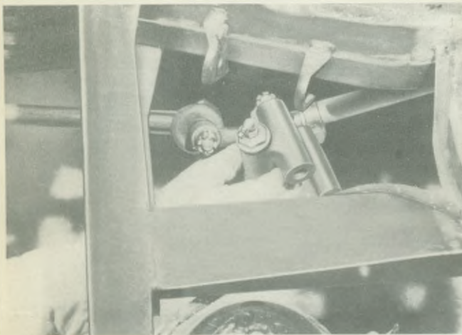
Fig. 26. Adjusting positing of auxiliary bracket to align centre tie rod with drop arm
