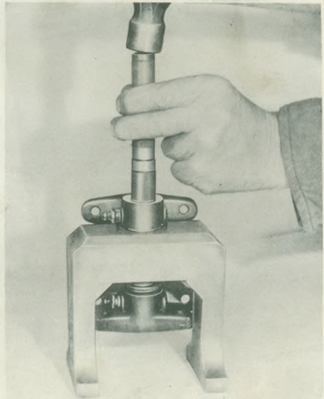
Fig. 11. Driving in swivel pin bushes with approved driver and locator
