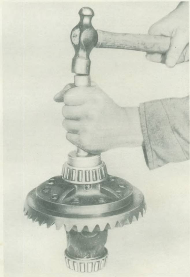
Fig. 19. Fitting inner ring of differential side bearing
