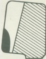
Fig. 31. Hypoid pinion tooth markings
