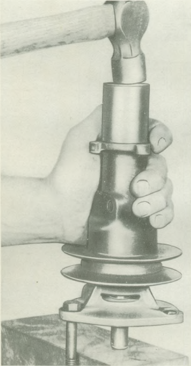
Fig. 5. Fitting fan extension bracket to bearing housing
