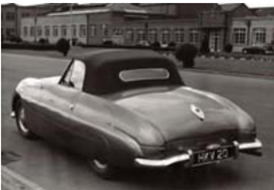
Below: the central filler cap became a tail motif. The bonnet could open to either side, and was also removable.
