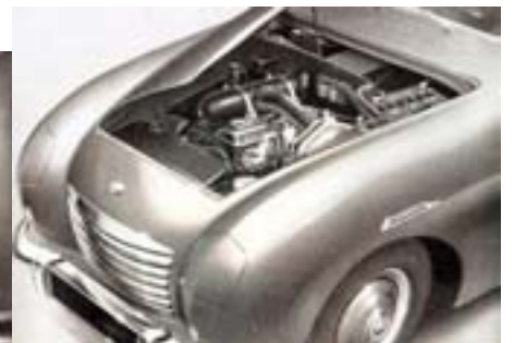
Below: the central filler cap became a tail motif. The bonnet could open to either side, and was also removable.
