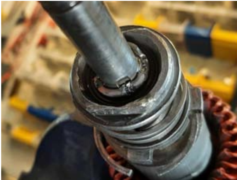
The February calendar picture - the mangled end of the starter armature Photo: Ian Dimmack
