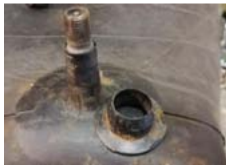
An old steel wheel - not one of Mike's - showing the central rivet-heads, and also the width of the deep central well into which the tyre bead can drop, if you drive with it completely deflated. This is less likely if you have tubed tyres.
