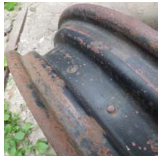
An old steel wheel - not one of Mike's - showing the central rivet-heads, and also the width of the deep central well into which the tyre bead can drop, if you drive with it completely deflated. This is less likely if you have tubed tyres.
