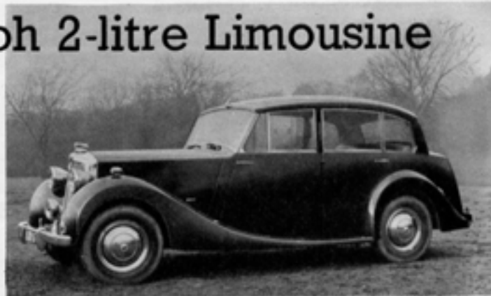
SMART CARRIAGE. —The dignified external lines of the 2-litre Triumph Limousine are similar to the better-known saloon model. Recently the wheelbase of the latter has been increased so that both types now use a similar chassis.
