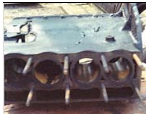
It’s not meant to have ventilation in the side...
