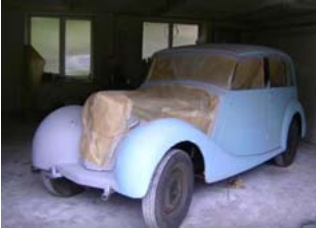
Wrapped and undercoated, then beginning the final paint finish. Yes, he's going for a bold two-tone.
