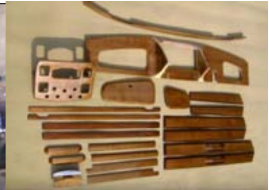
Above: all the wooden trim, cleaned and varnished – and in the case of the dashboard, built, veneered and varnished.
