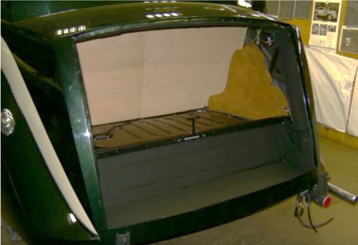
The re-lined boot area, showing the top of the petrol tank.
