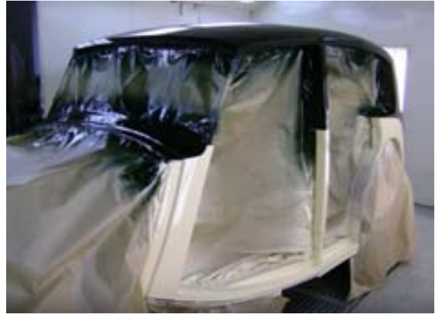
Wrapped and undercoated, then beginning the final paint finish. Yes, he's going for a bold two-tone.
