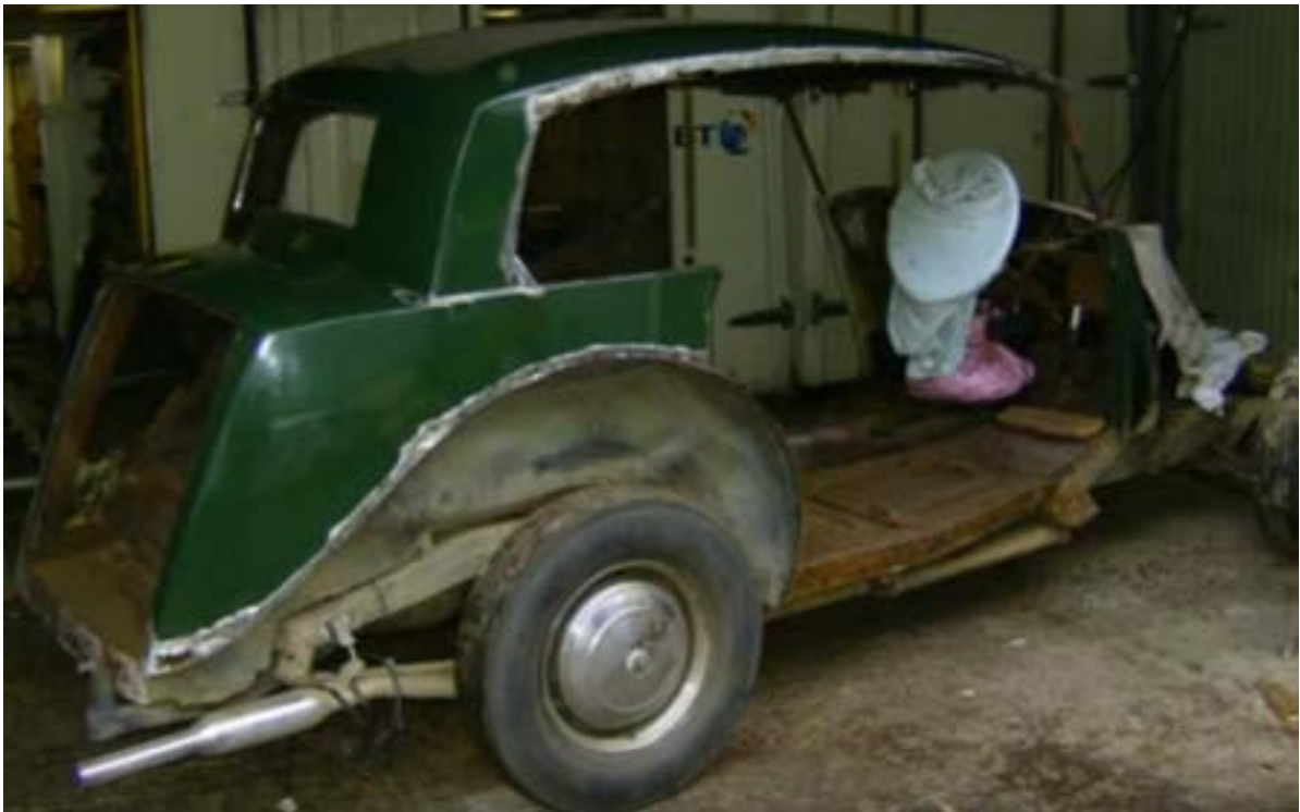
Door pillars and doors, rear bumper and valance, and windscreen off; engine and gearbox out.
