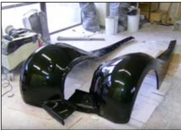
The wings and doors have been sprayed separately; then it's back onto the trailer on the way home, ready for re-assembly. Below, replacing the wiring loom and re-inserting the dashboard, ready for the instrument panel.
