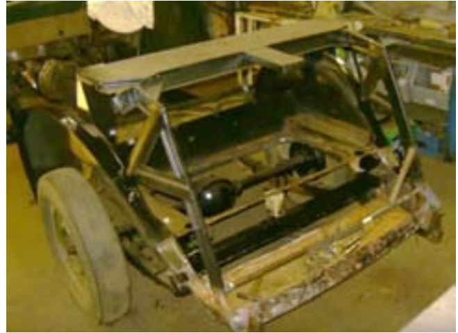
Showing the steering box, and the brake pipes including the brake lights operating switch covered in last month's Globe. Then the rebuilt rear of the car, petrol tank out, showing the axle and differential.
