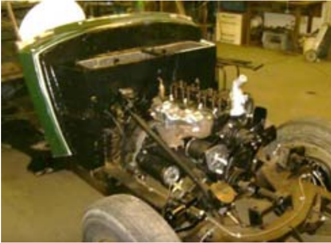
Showing the steering box, and the brake pipes including the brake lights operating switch covered in last month's Globe. Then the rebuilt rear of the car, petrol tank out, showing the axle and differential.
