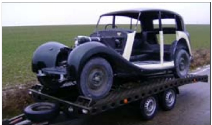
The wings and doors have been sprayed separately; then it's back onto the trailer on the way home, ready for re-assembly. Below, replacing the wiring loom and re-inserting the dashboard, ready for the instrument panel.
