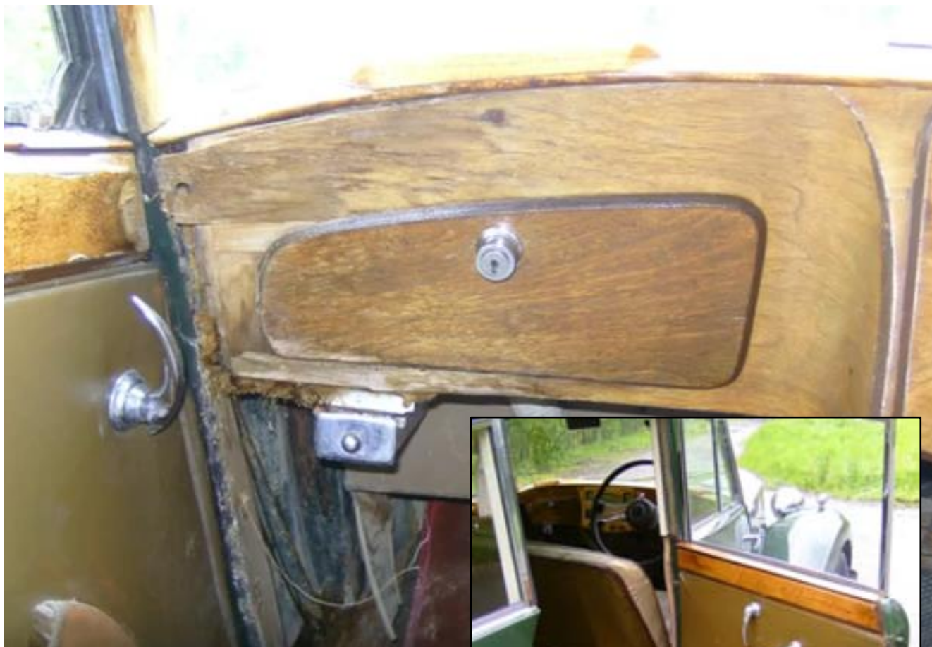
Ah yes; so it has. The side panel has also rotted and distorted.
