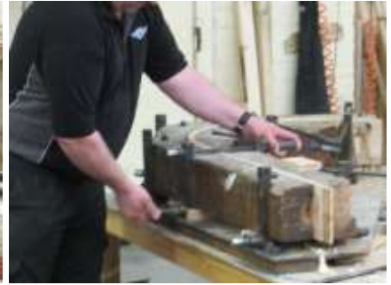
Three sheets of ply, freshly-glued, are bent into the mould to be clamped until set, making a wing.
