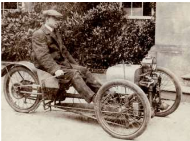
The Runabout, the first Morgan car, with HFS Morgan at the... tiller. Because of its light weight, it could accelerate as well as any car in production at that time.
