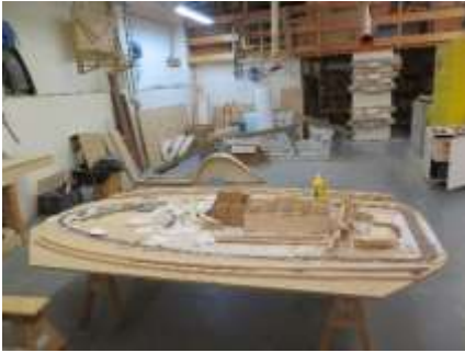
Three sheets of ply, freshly-glued, are bent into the mould to be clamped until set, making a wing.
