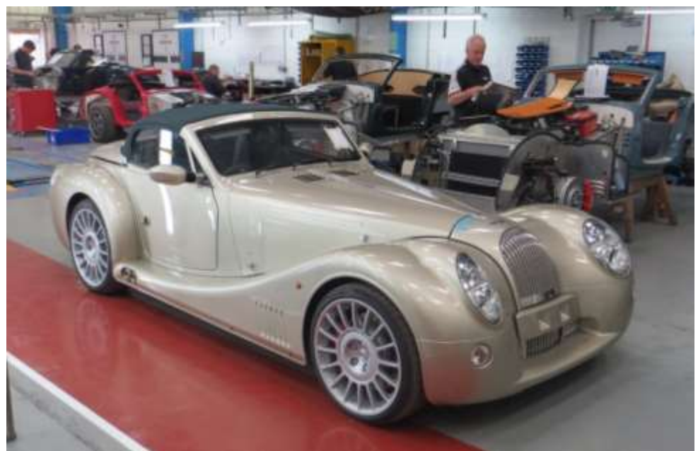
The bonnet is apparently one of the hardest parts to get right; because of variations in the wood frame and the scuttle position, the bonnet halves are all made over-size, rolled to the required curve, and then shaped individually.
