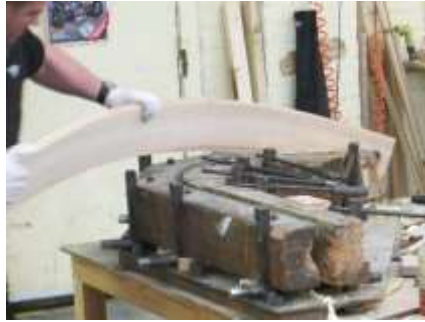
Three sheets of ply, freshly-glued, are bent into the mould to be clamped until set, making a wing.
