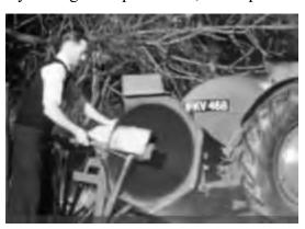
Fitted with a circular saw – and no safety guards!
