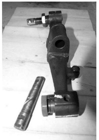
The photo shows the old vertical link with the bushes and fulcrum bolts. It is easy to see how worn the old fulcrum bolt is. The hairline cracks are marked with chalk.
