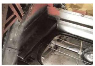
"All the woodwork has been remade and given 3 coats of clear Sadolin. The chassis has been taken down to bare metal, repaired, and then new bushes fitted. It has had 3 coats of Hammerite, and finally Waxoyled inside. All steering, springs, suspension and brakes parts have been given similar treatment.
