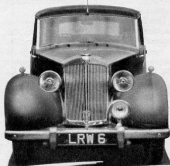
TRADITIONAL LINES have a functional aspect, both side-lamps being visible to the driver through the large windscreen.
